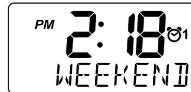
4. Rotate the Tuning control to choose the required alarm type, and then press and release the Tuning control to confirm the setting. The alarm can be set to buzzer, iPod, FM or AM. When radio mode is selected, the radio frequency and the preset number on the display will begin to flash. Rotate the Tuning control to adjust the required radio frequency or the required preset number for the radio alarm, then press and release the Tuning control to confirm the setting.
