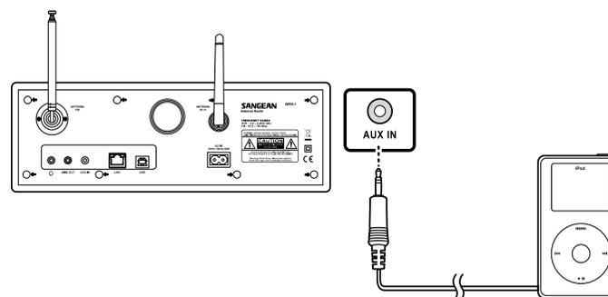
2. Go to >Main menu>Auxiliary input or press AUX IN on the remote.
