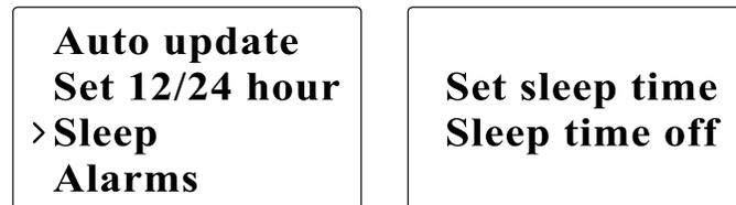
2. Use TUNE+/TUNE- or Turning knob to toggle between off, 15 minutes, 30 minutes, 45 minutes, and 60 minutes.
